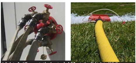
Left photo: Capti Fire pump test header set up for full flow testing. Right photo: Little Hose Monster diffusing water flow during flow testing.
